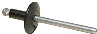
3/16 SIZE .12 - .25 PANEL .62 OD OIU, 6033249 ALL ALUMINUM BLACK ANODIZED
